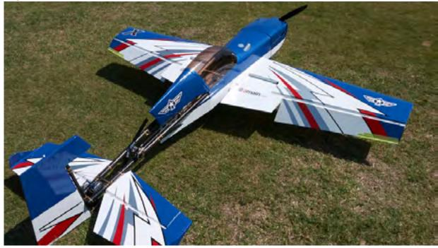
We saw this unique plane at the 3D line at Joe Nall. Called the "Super Honey Badger." It is unique in that it has a helicopter rotor towards the tail. A separate motor turns the rotor blade and the pitch can be changed via the radio. Talk about flat spins. Amazing to watch.
