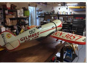
It is 85" span and for a 45-50cc gas engine, his has an EME 55 gas with on-board electric starter system.
